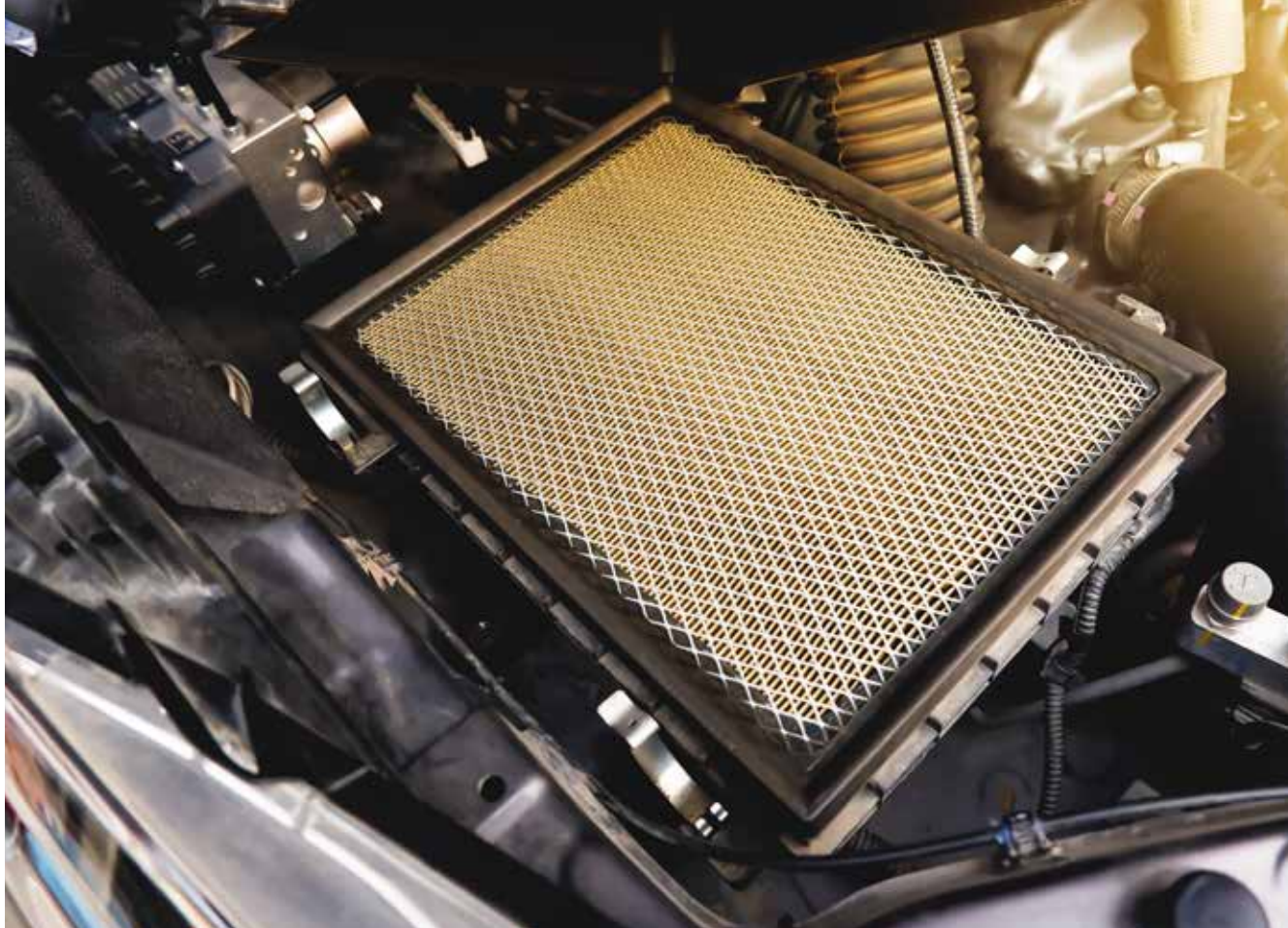
Cabin or engine air filters often contain expanded metal to support the paper or fleece media
